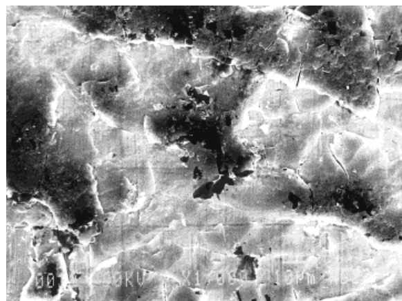
Figure 10 Scanning electron micrograph of the copper side in the PI/3070/Cu sample with preoxidation of the primer after the peel test.
